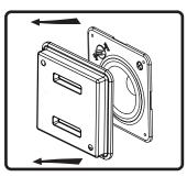
**8.** Remove paint mask unless painting is required. In that case, follow steps 9-12 when painting is complete.
